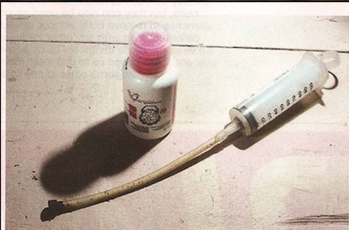
Effetto Mariposa sealant injector: This oversized syringe makes it easy to measure and inject sealant into any Presta tubeless valve. It comes with a thread-on fitting to prevent spills and comes with gradients to be sure the volume of sealant you're installing is precise and consistent.
